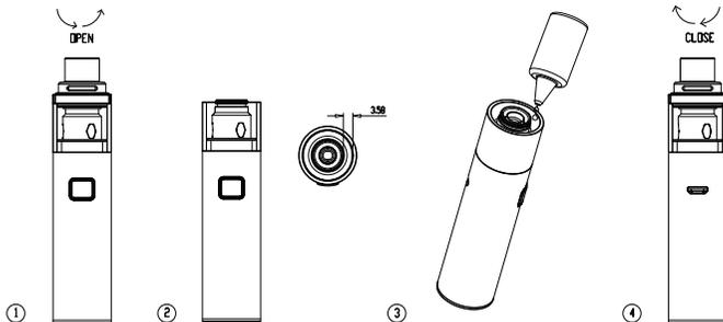
**4. Changing Atomizer:** Unscrew the tank from the base to remove and insert a new atomizer. Pull the EUC out from the base and insert a new one. Screw the Base on. Wait after replacing to make sure the coil is well primed.
